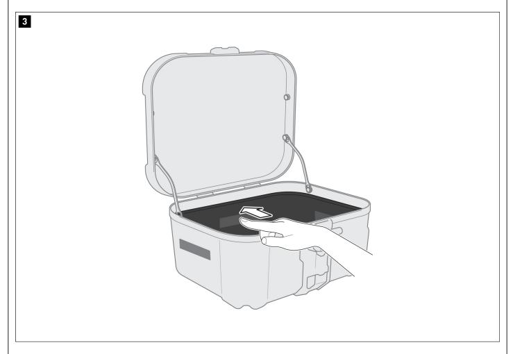
$\dots$  and press the inlay (1) against the wall of the DUSC. Make sure the inlay (1) is held firmly in place.
