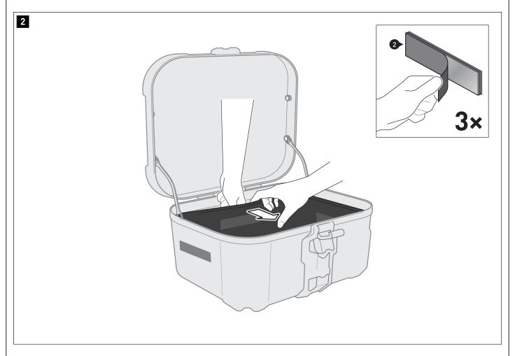
Once the inlay (1) is in place, carefully pull the sides of the inlay (1) away from the wall of the DUSC.
